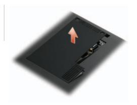
Remove the back cover to access the FCM or WWAN Mini Card slot to install the Latitude ON Flash card.
